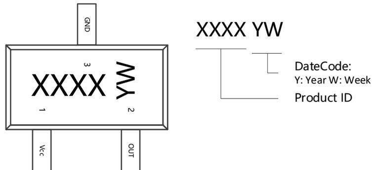
Figure.15 SOT-23 Chip Marking Spec
