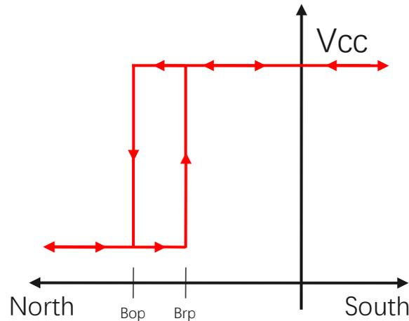
**Figure.2** Switching Function Uni-polar (North)
