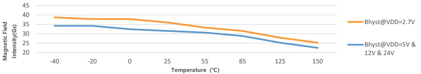
Figure.8 Magnetic Characteristics vs. Temperature &  $V_{DD}$  ( $B_{HYST}$ )
