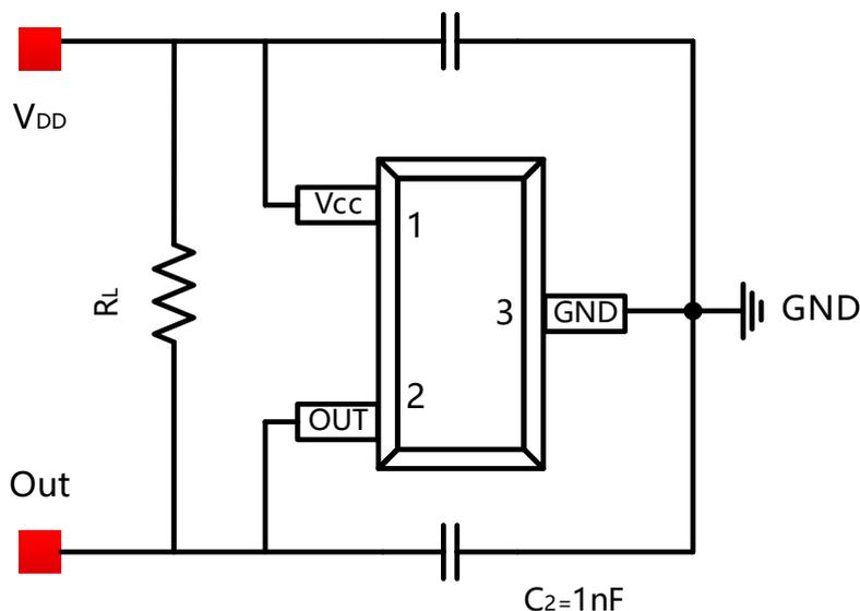
Figure.12 Typical Application Circuit (MT8911AT as example)
