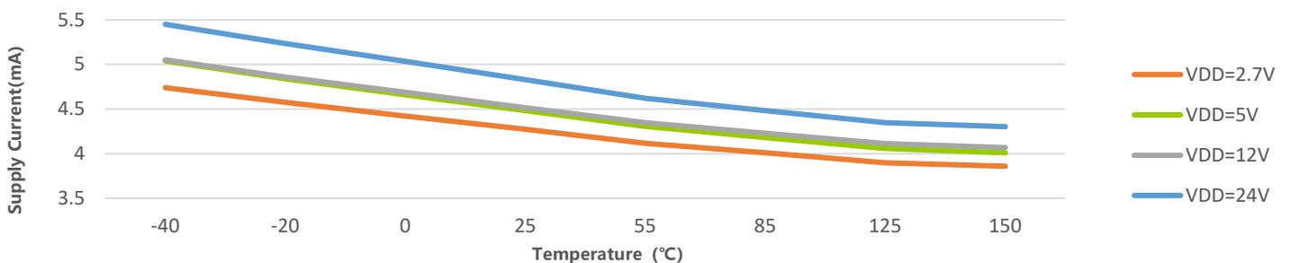
Figure.6 Supply Current vs. Temperature &  $V_{DD}$
