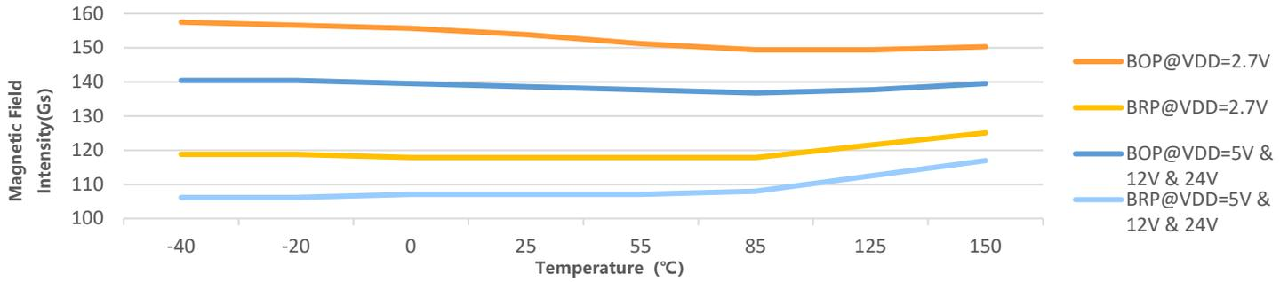
Figure.7 Magnetic Characteristics vs. Temperature &  $V_{DD}$  ( $B_{OP}$  &  $B_{RP}$ )
