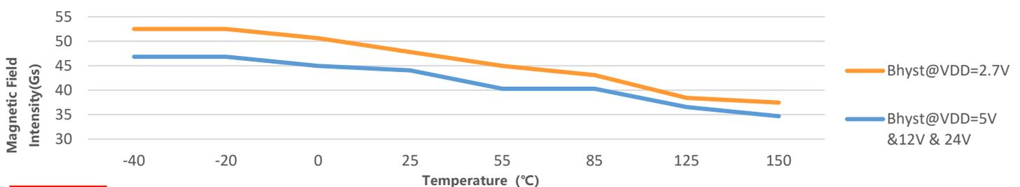
Figure.11 Magnetic Characteristics vs. Temperature &  $V_{DD}$  ( $B_{HYST}$ )
