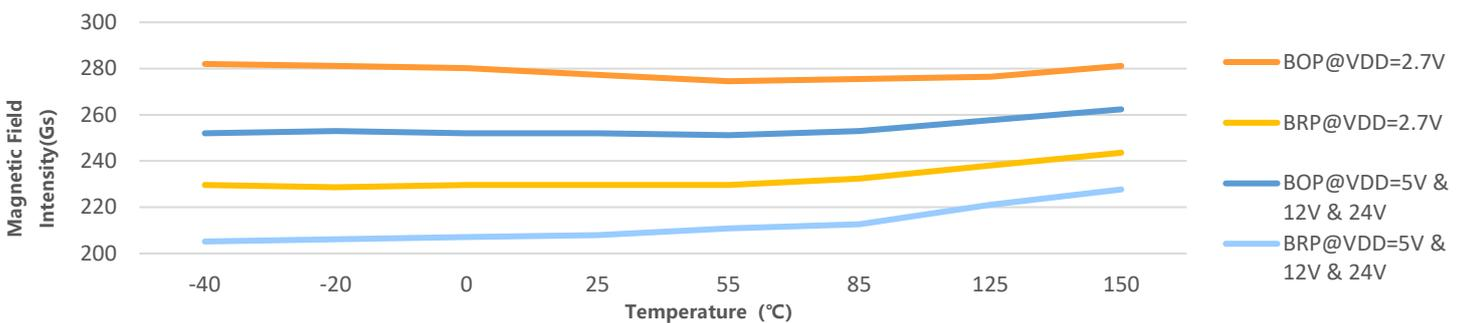
Figure.10 Magnetic Characteristics vs. Temperature &  $V_{DD}$  ( $B_{OP}$  &  $B_{RP}$ )
